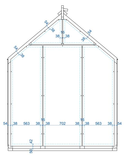
NB! Make sure that the glasses are evenly spaced and that the attachment points line up. Observe the alignment of the glasses at their lower edge. The lower edge of the back wall glass must be 50 mm from base frame elements gap and line up with side glass lower edge.
