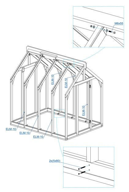
NB! Tighten the nuts only later after installing the rafter middle details! (Look section 13)
