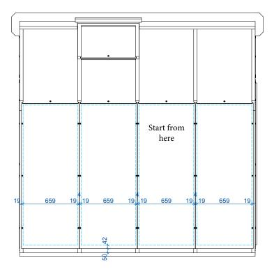
NB! Make sure that the glasses are evenly spaced and that the attachment points line up. Observe the alignment of the glasses at their lower edge.
