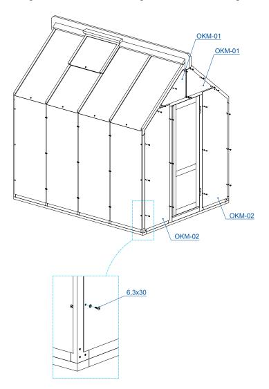
NB! Make sure that the glasses are evenly spaced and that the attachment points line up. Observe the alignment of the glasses at their lower edge. The lower edge of the back wall glass must be 50 mm from base frame elements gap and line up with side glass lower edge.
