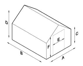
Roof pitch – 40° Snow load – 250 kg/m2 Sidewind load – 45 kg/m2
