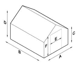
Roof pitch - 16° Snow load - 250 kg/m2 Sidewind load - 45 kg/m2
