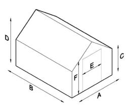
Roof pitch - 36° Snow load - 250 kg/m2 Sidewind load - 45 kg/m2
